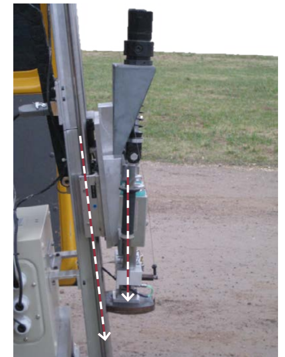
▲ The metal “hoof” is mounted beneath a heavy weight, which is dropped to the ground between two guide rails. The rails have different angles, which mimics the motion of the early landing/touchdown phase, as a simultaneous downward motion and forward slide of the ‘hoof’ occurs when it contacts the ground.
