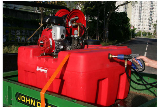
Fig. 6. A mobile cooling unit. A 400 L tank with integral petrol engine-driven pump was mounted on the back of an agricultural 4-wheel-drive utility vehicle.
